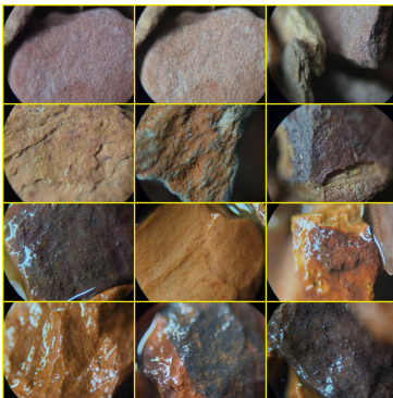
Figure 27: Microscopic Analysis of Seachem Flourite. Comparison of unused (top/middle) and used (bottom) granules. No visible structural alteration; particles remained intact. (Brightfield, 100× magnification).
