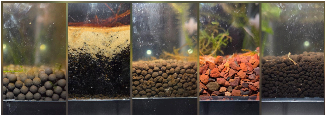
Figure 22: Final Substrate Appearance in Situ (Day 148). Close-up views of each substrate bed. Note the layering and compaction in the Organic Compost tank (second from left). Lower samples are freshly wet, photographed immediately after removal.
